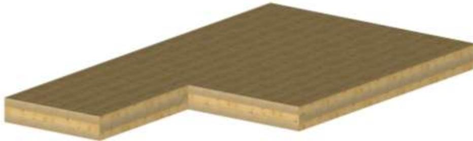
Figure 2 Layout of a 3-ply CLT panel.
